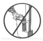
draught can be helped by blowing air to the opening of the air slide or by burning a small firelighter in the upper part of the chimney. The mouth of the stove and the hatch will bend if you let the draught continue in the wrong direction. **This will not be covered by the guarantee**.
